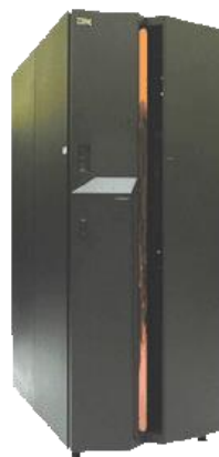
IBM P690 256 CPU's/ 768 Gflops
