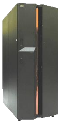
IBM P690 A 96 CPU's/ 729.6 Gflops
